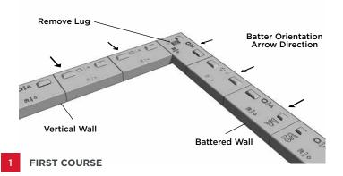
Combination corners have a Battered wall on one side and Vertical wall on the other. This is ideal for step side walls to eliminate difficult cuts.
