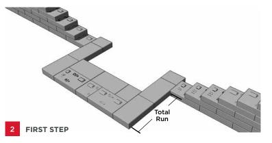
Start the wall with two inside 90° Combination corners (page 11) and two outside 90° corners using closed-end coping blocks. Use the Total Run formula to determine the distance out from the face of the wall where the front of the first riser should be placed. Place another row of Stardard Coping blocks directly behind the first set.
