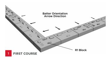
When constructing a Battered Retaining Wall, Alternate between R1 & R2 blocks for each course. At the corner location, place an R1 block as shown. Abut a standard block next perpendicular to the R1 block, ensuring the Batter Indicator is pointing Forward. Continue to install standard blocks as shown with the Batter Indicators pointing Forward.
