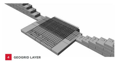
Experience has shown that the inclusion of geogrid reinforcement within each course of steps reduces the effect of settlement. It is recommended to include an additional geogrid layer every other step placed in the perpendicular principle direction.
