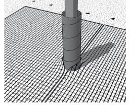
To place the sonotubes, cut the geogrid perpendicular to the wall along the centerline of the sonotube, creating two geogrid panels one on each side of the sonotube. Lay the geogrid flat in front of the sonotube. At the intersection with the sonotube, fold the geogrid flat against vertical side of the sonotube and then around the back, maintaining the edge of the geogrid along the centerline of the sonotube. Lay the geogrid flat behind the sonotube and pull taut.
