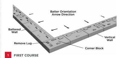
Combination corners have a Battered wall on one side and Vertical wall on the other, this is ideal for step side walls to eliminate difficult cuts.
