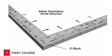
Vertical walls are constructed by utilizing ALL V1 or ALL V2 Blocks for each course.
