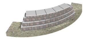
The ReversaCap coping units can be placed with the wide face positioned the same way to create a curve. If the radius is greater or less than 2.4m (8ft), the ReversaCap coping units will require several cuts to create a continuous top surface.
