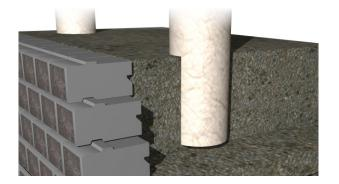
Cut the geogrid perpendicular to the wall along the centerline of the sonotube, creating two geogrid panels - one on each side of the sonotube. Lay the geogrid flat in front of the sonotube. At the intersection with the sonotube, fold the geogrid flat against vertical side of the sonotube and then around the back, maintaining the edge of the geogrid along the centerline of the sonotube.
