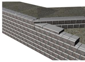
Continue constructing the upper wall and place the last standard course and coping on the lower wall. This will require a cut where this course abuts the beginning of the upper wall to ensure a tight fit.
