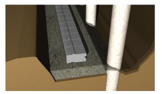
Construct the conventional SRW, stacking units and backfilling with drainage material. The recommended drainage material (¾ in clear stone) should be lightly compacted with a hand tamper, ensuring proper confinement around the sontotube.
