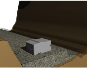
Identify the proposed location of the handrail foundations (sonotubes). Take into account the batter (setback) of the wall (19mm [¾in] per course) and the required offset at the top. It is preferable to leave a 300mm (12 in) buffer zone between the outside of the sonotube and the back of the wall. If this is not possible, expansion joint material must be placed between the back of the coping unit and concrete sonotube.
