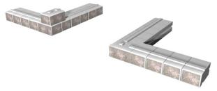
Build each wall up. The side walls can be built in either battered or vertical arrangement, as specified in the design. The side walls can be stepped up following the steps, but the side of riser (step) units must be in contact with the face of units in the side wall.
