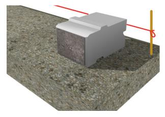
Ensure units are level front to back and left to right. Extra care should be taken at this stage as it is critical for accurate alignment.
