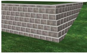
The wall could be abutted to an existing structure. This would involve cutting the retaining wall units in order to maintain the running-bond pattern. An expansion joint (25mm asphaltimpregnated fibreboard) should be constructed between the retaining wall and the structure.
