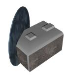
Score the top and bottom of the opposite side of the unit to a depth of approximately 12mm (0.5 in) at a 45° angle. The score line starts 200mm (7.87 in) from the rear of the unit.
