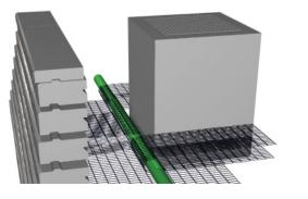
Select an appropriately sized steel pipe with a length of at least twice the width of the catch basin. Extend the geogrid from the specified layer and wrap it around the pipe back to the course below. Place a width of geogrid reinforcement (half the catch basin width) on either side of the catch basin, wrap around the pipe and extend into the infill material. Ensure that the geogrid extends the distance into the infill material as specified in the design.
