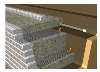
The loads produced by terraced walls can be great. As an example, a small 0.6m (2.0ft) high wall produces a load equivalent to a heavy traffic surcharge on the lower wall.
