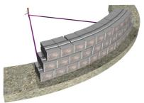
Geogrid layers should be placed within 25mm (1in) of the front face of the block. The geogrid will overlap and should have 75mm (3in) of compacted soil between the layers. The geogrid should be placed on the Pisa units so the geogrid does not overlap until it enters the soil zone.
