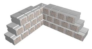
The geogrid should be placed within 25mm (1in) of the face of the block. As it is only necessary to have geogrid extending directly away from the wall, a gap will result in the geogrid layer as shown.
