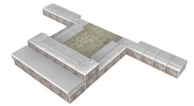
Continue to finish the second course of the wall. The side walls can be built in either battered or vertical arrangement as specified in the design. If the side walls are designed to be battered, each riser will be 38mm (1.5 in) narrower than the course below.
