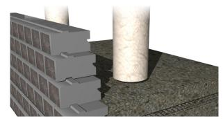
required offset at the top (It is preferable to leave a 300mm [12 in] buffer zone between the outside of the sonotube and the back of the wall. If this is not possible, expansion joint material must be placed between the back of the coping unit and concrete sonotube).
