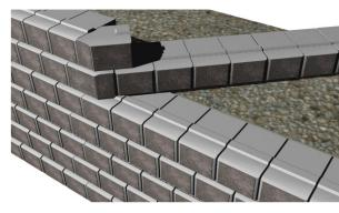
Prepare the base for the upper wall at the required angle or curve. As this offshoot wall will be resting partially on the existing lower wall and partially on the new base, the potential for differential settlement exists. Extra care must be taken to ensure the Wall 2 base has been properly compacted to 98% SPD. As this base is bearing on the reinforced zone of the lower wall, construction of this area is vital.
