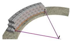
Geogrid layers should be placed within 25mm (1in) of the front face of the block. It will be necessary to have gaps between adjacent sections of geogrid. At alternating geogrid elevations the geogrid sections should be positioned so they overlap the gaps in the geogrid on the layers below.
