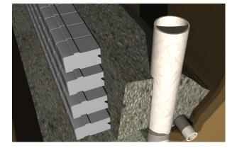
Secure the coping unit and fold filter cloth back over drainage material. Cut filter cloth at centerline of sonotube to allow the sonotube through, ensuring complete coverage of drainage material. Cover sonotubes prior to concrete pour to prevent debris from entering.
