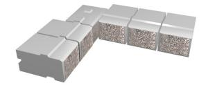
Commence second course by placing alternate corner unit to interlock corner.
