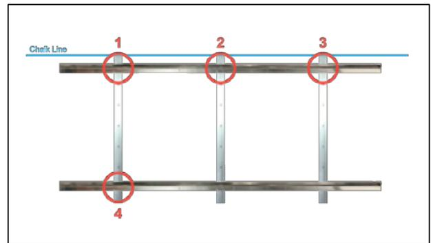
**Step 3:** Fasten the bottom horizontal rail and alignment bar at point 4; use a level or a square to ensure alignment bar is plumb
