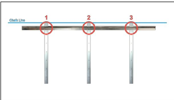
**Step 2:** Fasten both horizontal rail and alignment bars to substrate at points 1, 2, and 3; ensuring the rail is level.
