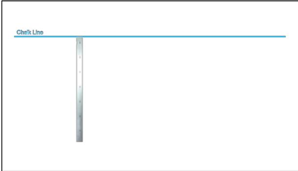
**Step 1:** Determine finished top height, mark with chalk line. Align orange painted end of alignment bar with chalk line.
