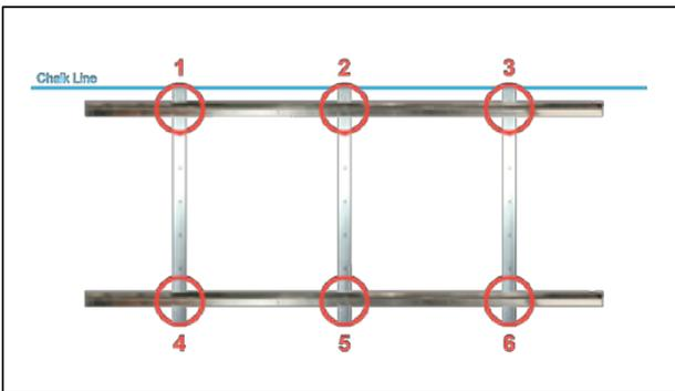
**Step 4:** Fasten the bottom horizontal rail and alignment bars at points 5 and 6.
