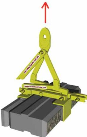
Place unit in desired location. Once set in place, rotate locking bar back to centre peg. This restrains the clamp from closing. Lift clamp away from block.
