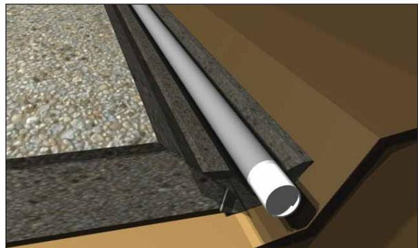
In the case of connecting to a positive outlet, the drain should be placed at the lowest possible elevation and sloped at a minimum of 2%. At the rear of the base, allow the granular material to slope down on the sides towards the drain trench. In the 185mm (7.25 in) area behind the base, place the approved drain tile (perforated drain with filter sock) on top of the filter cloth and minimal granular coverage.
