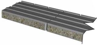
Continue placing base course units on adjacent wall. A half-unit overlap will be required as shown to maintain the running bond pattern.
