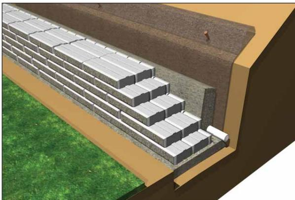
The minimum dimensions of the 925 unit granular base are 1295mm (51 in) wide (front to back) and 185mm (7.25 in) deep.
