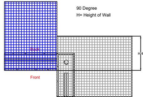
Note: Geogrid should be placed to avoid any overlapping between blocks.
