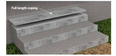
Tip: Whenever possible install full length pieces for the tread. Short coping units must have grouted joints. Grouted joints on stairs have a limited life before they need repair.
