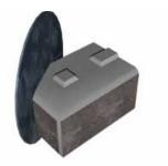
Score the top and bottom of the opposite side of the unit to a depth of approximately 12mm (0.5 in) at a 45° angle. The score line starts 200mm (7.87 in) from the rear of the unit. Using a chisel and hammer, break off the corner of the unit to reveal a rock-faced 45° unit.
