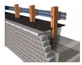
Proper drainage of a segmental retaining wall is one of the most critical aspects of design and construction. Unless otherwise stated, the design assumes that no hydrostatic pressures exist behind the wall. To ensure this condition is met, water flow from all directions and sources must be accounted for in the design through proper grading and drainage measures, diverting water away from the wall whenever possible.
