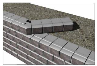
The low wall (Wall 1) must be designed based on the maximum height required. As Wall 1 splits into an upper (Wall 2) and lower wall, the lower wall must still be designed for the additional loading until the point where the upper wall has diverged far enough back to reduce the effect.
