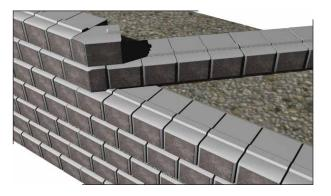
Prepare the base for the upper wall at the required angle or curve. As this offshoot wall will be resting partially on the existing lower wall and partially on the new base, the potential for differential settlement exists. Extra care must be taken to ensure the Wall 2 base has been properly compacted to 98% SPD. As this base is bearing on the reinforced zone of the lower wall, construction of this area is vital.
