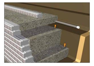
The loads produced by terraced walls can be great. As an example, a small 0.6m (2.0ft) high wall produces a load equivalent to a heavy traffic surcharge on the lower wall. These loads may be reduced by increasing the offset between the walls or increasing the foundation depth of the upper wall. Wherever possible, the lower wall should be higher than the upper wall.
