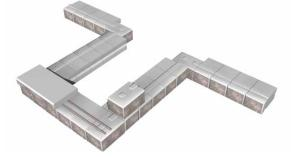
Place the next riser on the base with the face of units in contact with the back of the coping units at the first riser. Some chopping will be necessary for the positioning of left and right corner units.
