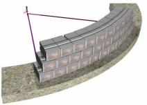
Geogrid layers should be placed within 25mm (1 in) of the front face of the block. The geogrid will overlap and should have 75mm (3 in) of compacted soil between the layers. The geogrid should be placed on the Pisa2 units so the geogrid does not overlap until it enters the soil zone.
