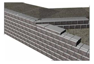
Continue constructing the upper wall and place the last standard course and coping on the lower wall. This will require a cut where this course abuts the beginning of the upper wall to ensure a tight fit.
