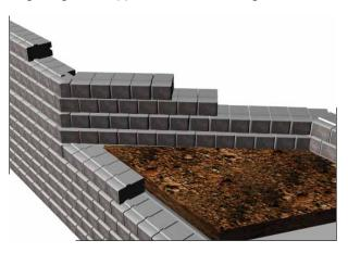
Place filter cloth in the area between the upper and lower walls, ensuring the required reinforced zone of the lower wall and base of the upper wall are adequately protected. Grade as required.
