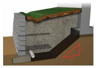
The Pisa2 system offers the flexibility to create a wide variety of step configurations and designs. As with any SRW structure, proper base preparation is critical to success when constructing steps. We recommend that only a free-draining, well-graded, granular material be used for the 150 mm (6 in) base at each riser. Compaction at each step (to 98% SPD) is crucial to resisting settlement due to continuous pedestrian loading.
