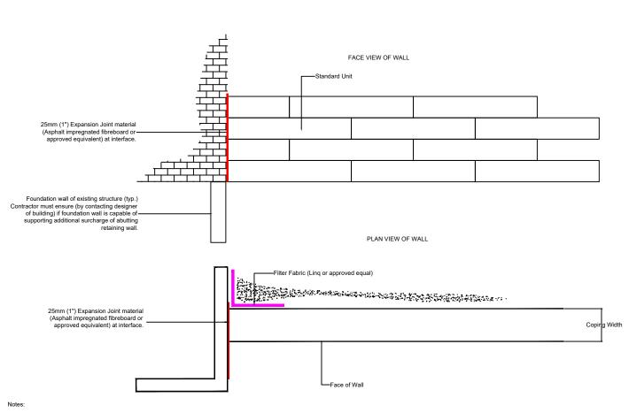
1. Retaining Wall and existing abutting structure must remain structurally independent.
