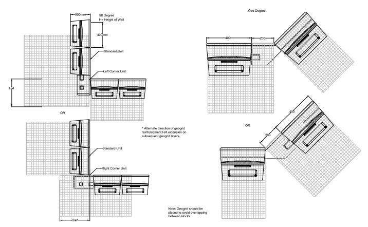
Note: Geogrid should be placed to avoid overlapping between blocks. In order to compensate for the left out area place Geogrid on the next course (at left out area only). Geogrid to block spacing per design.
