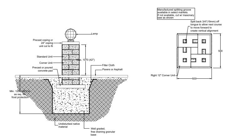
Note: Poor site conditions can affect the stability of the structure. Consult a qualified professional engineer to determine site specific construction details.
