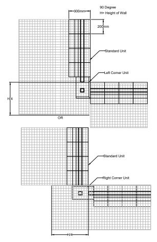
Note: Geogrid should be placed to avoid overlapping between blocks.
