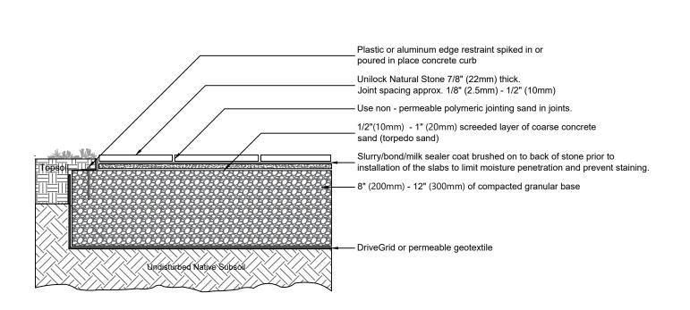
Important Note: Traditional Sand Set is an older method of installation and may result in bleed-through staining and/or efflorescence. It should only be used in warm, dry climates.
