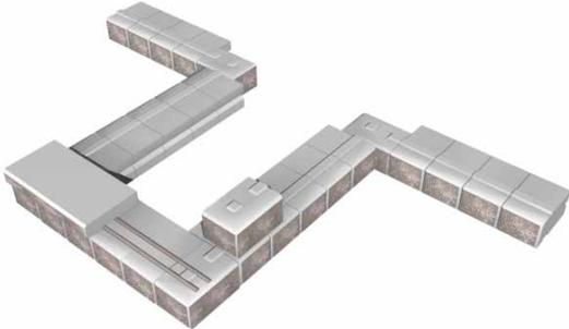
Place the next riser on the base with the face of units in contact with the back of the coping units at the first riser. Some chopping will be necessary for the positioning of left and right corner units.
