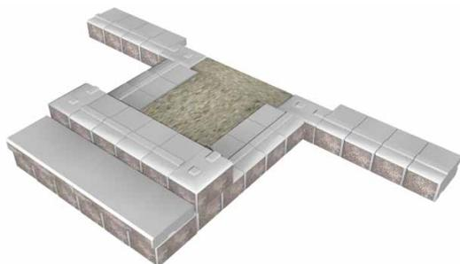
Continue to finish the second course of the wall. The side walls can be built in either battered or vertical arrangement as specified in the design. If the side walls are designed to be battered, each riser will be 38mm (1.5in) narrower than the course below.
