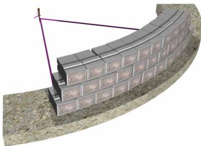
Geogrid layers should be placed within 25mm (1 in) of the front face of the block. The geogrid will overlap and should have 75mm (3 in) of compacted soil between the layers. The geogrid should be placed on the Pisa2 units so the geogrid does not overlap until it enters the soil zone.
