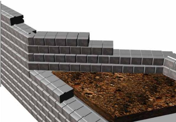
Place filter cloth in the area between the upper and lower walls, ensuring the required reinforced zone of the lower wall and base of the upper wall are adequately protected. Grade as required.
