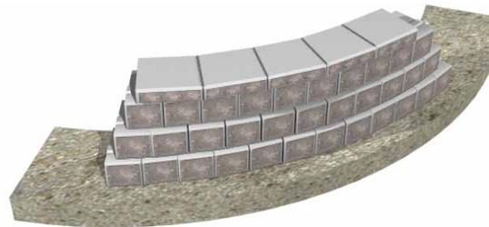
The ReversaCap coping units can be placed with the wide face positioned the same way to create a curve. If the radius is greater or less than 2.4m (8ft), the ReversaCap coping units will require several cuts to create a continuous top surface.
