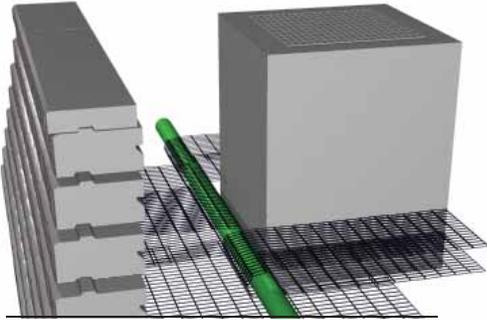
Select an appropriately sized steel pipe with a length of at least twice the width of the catch basin. Extend the geogrid from the specified layer and wrap it around the pipe back to the course below. Place a width of geogrid reinforcement (half the catch basin width) on either side of the catch basin, wrap around the pipe and extend into the infill material. Ensure that the geogrid extends the distance into the infill material as specified in the design.
