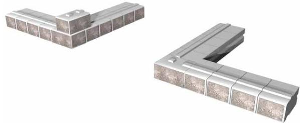
Build each wall up. The side walls can be built in either battered or vertical arrangement, as specified in the design. The side walls can be stepped up following the steps, but the side of riser (step) units must be in contact with the face of units in the side wall.
