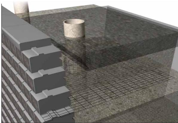
Pour concrete in foundations in accordance with fence/handrail design (reinforcing steel and/or dowels may be required). Install fence and finish grading.
