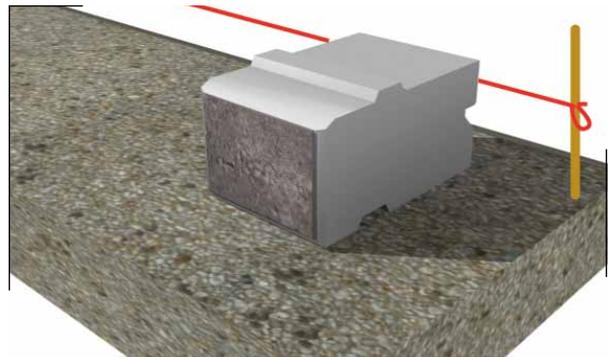
Ensure units are level front to back and left to right. Extra care should be taken at this stage as it is critical for accurate alignment.
