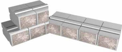
Cut left corner at desired angle, leaving  $\frac{1}{4}$  of the face, and place standard units to complete the course.
