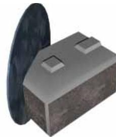
Score the top and bottom of the opposite side of the unit to a depth of approximately 12mm (0.5 in) at a 45° angle. The score line starts 200mm (7.87 in) from the rear of the unit. Using a chisel and hammer, break off the corner of the unit to reveal a rock-faced 45° unit.
