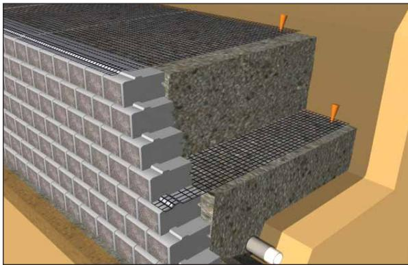
Backfill next lift of granular infill material on top of the geogrid reinforcement, placing the loose material at the front of the wall, and raking it back, away from the face (this method maintains tension in the geogrid during backfilling). Continue stacking and backfilling until the next layer of geogrid reinforcement is reached.
