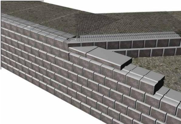
Continue constructing the upper wall and place the last standard course and coping on the lower wall. This will require a cut where this course abuts the beginning of the upper wall to ensure a tight fit.
