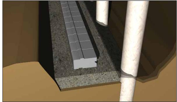
Construct the conventional SRW, stacking units and backfilling with drainage material. The recommended drainage material (¾ in clear stone) should be lightly compacted with a hand tamper, ensuring proper confinement around the sonotube.
