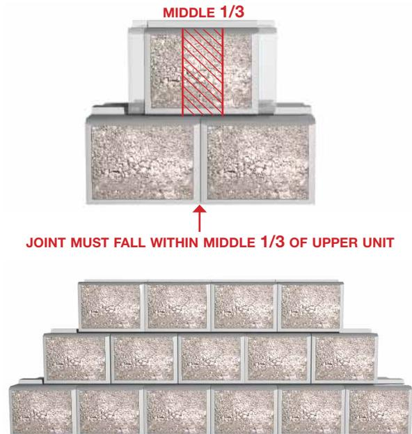
*[Note: When certain details – such as corners and curves – are incorporated into the wall, the running bond pattern may shift slightly. A small deviation from the perfect running bond pattern is allowable. However, this deviation should be corrected as soon as the wall layout allows.]*
