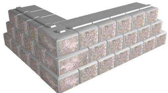
The geogrid from the two side walls will overlap and should be separated by a minimum of 75mm (3 in) of compacted soil. Alternatively, the geogrid reinforcement could be placed in the perpendicular principle direction in the cross-over area on the succeeding course.
