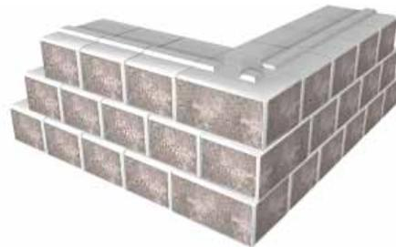
Place the first course of step units on the same foundation elevation as the side walls. A unit may have to be cut to make the riser fit between the side walls. Fill in base materials at the back of the riser and make it even with the top of the first course. The coping is then cut (if necessary), positioned, and secured with an adhesive.
