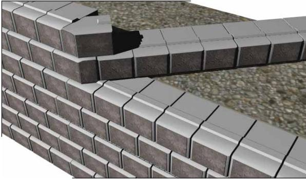
Prepare the base for the upper wall at the required angle or curve. As this offshoot wall will be resting partially on the existing lower wall and partially on the new base, the potential for differential settlement exists. Extra care must be taken to ensure the Wall 2 base has been properly compacted to 98% SPD. As this base is bearing on the reinforced zone of the lower wall, construction of this area is vital.
