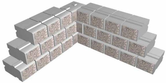
The geogrid should be placed within 25mm (1 in) of the face of the block. As it is only necessary to have geogrid extending directly away from the wall, a gap will result in the geogrid layer as shown.
