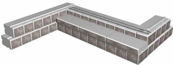
Repeat the previous stage to finish the third course. Use a left corner unit at the inside corner this time. At the riser, one unit may have to be cut to fit in.
