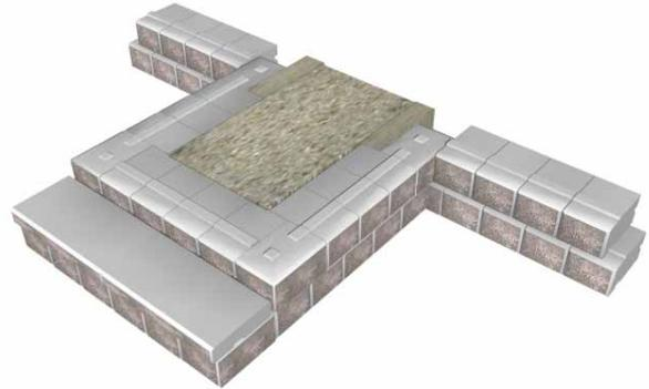
Repeat the above steps to finish the wall. However, units may have to be cut to fit in the side wall.
