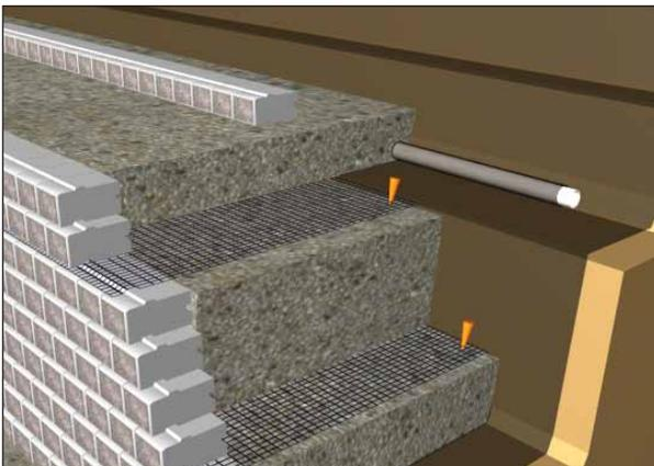
The loads produced by terraced walls can be great. As an example, a small 0.6m (2.0ft) high wall produces a load equivalent to a heavy traffic surcharge on the lower wall. These loads may be reduced by increasing the offset between the walls or increasing the foundation
