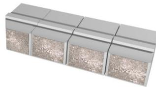
Cut right corner off adjacent unit at the same angle, leaving ¼ of the face, and continue placing base course units on adjacent wall.
