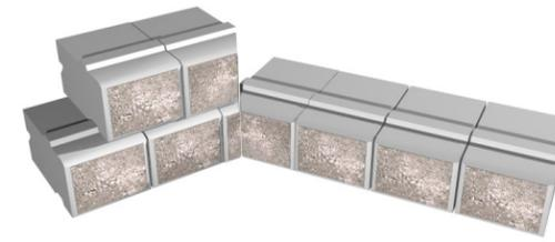
Cut left corner at desired angle, leaving ¼ of the face, and place standard units to complete the course.
