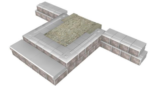
Repeat the above steps to finish the wall. However, units may have to be cut to fit in the side wall.
