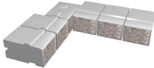
Commence second course by placing alternate corner unit to interlock corner.
