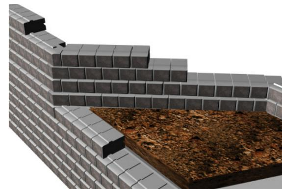
Place filter cloth in the area between the upper and lower walls, ensuring the required reinforced zone of the lower wall and base of the upper wall are adequately protected. Grade as required.
