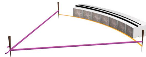
material and compact to 98% SPD. The top elevation of the base should be flush with the top elevation of lower units. The face of riser units must be in contact with the back of the coping units on the lower course. Make sure the new curve is parallel to the curve of lower riser.
