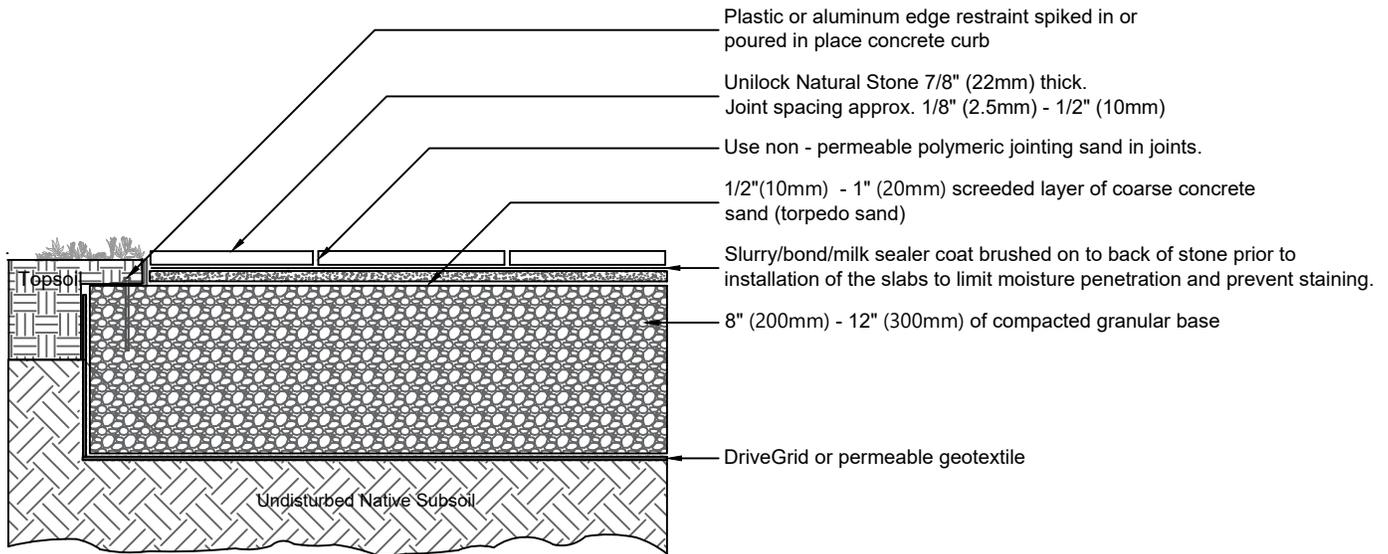
Important Note: Traditional Sand Set is an older method of installation and may result in bleed-through staining and/or efflorescence. It should only be used in warm, dry climates.
