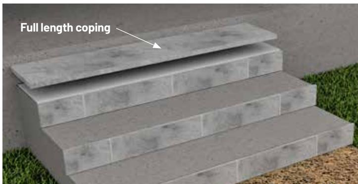
➤ **Tip:** Whenever possible install full length pieces for the tread. Short coping units must have grouted joints. Grouted joints on stairs have a limited life before they need repair.
