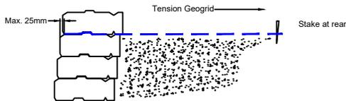
Step 4. Place infill material near face of wall and spread back, away from wall to maintain geogrid tension. Compact infill material in max. 150mm-200mm (6"-8") lifts. Continue process to next geogrid layer.
