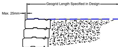
Step 3. Secure geogrid in place at face with next course and pull geogrid taut. Maintain tension with temporary stakes as shown.
