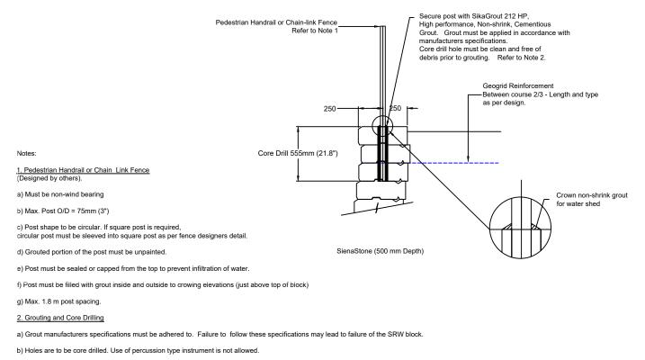
c) Core drill hole to extend completely through the specified number of courses to allow high pressure water jet (or other suitable means) to clean hole of dust and debris prior to grouting.
