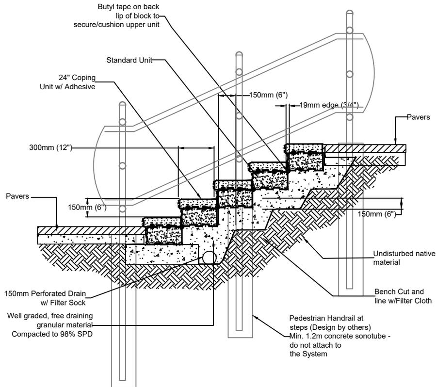
Note: Poor site conditions can affect the stability of the structure. Consult a qualified professional engineer to determine site specific construction details.
