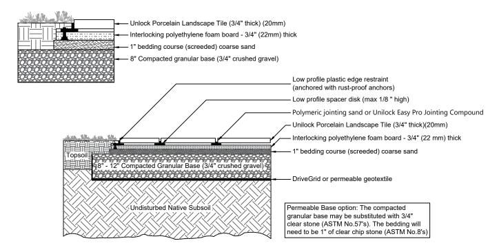
Note: Expanding polyethylene foam board (EPFB) facilitates the rapid installation of porcelain paving slabs. Although foam board distributes load, it is important that the are below the board has good load bearing capacity and provides sufficient drainage to keep the area below free of any frost movement. Only use EPFB's manufactured for this application, not recommended for vehicular applications.
