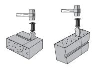
To split a large convertible unit, use a hammer and chisel to score the top and sides, then lip the unit upside down and use the chisel to break the unit. This may require a couple of hits along the groove to achieve a clean break.
